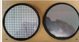
(a) 4 inch 1,700 volt SiC Junction Barrier Schottky diodes wafer (16x5 mm 2 chips), (b) 4 inch 4,500 volt SiC pin-diode (2.5x2.5 mm 2 chips) wafer. Both developed at ABB Corporate Research.
