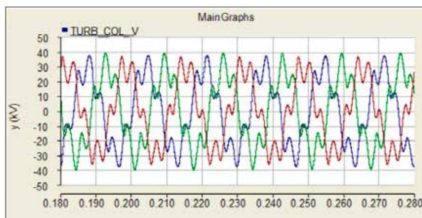
Figure 2. Collector system overvoltages from the wind generation harmonic spectrum [2]
