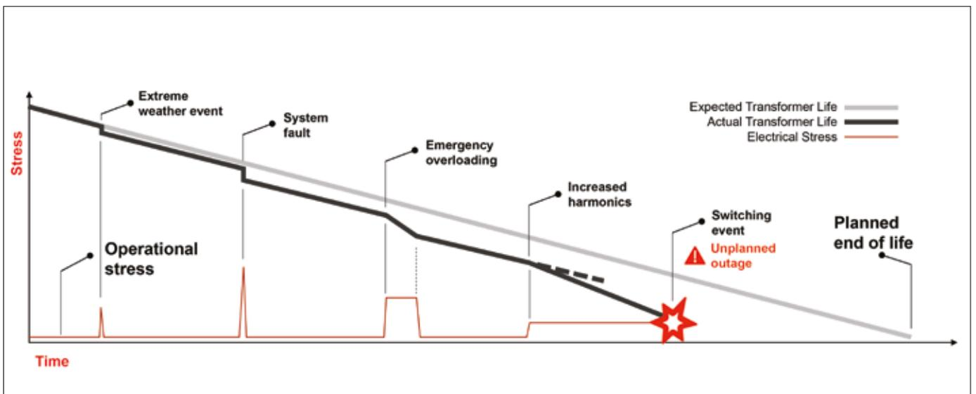
Figure 4. Typical transformer stress events
