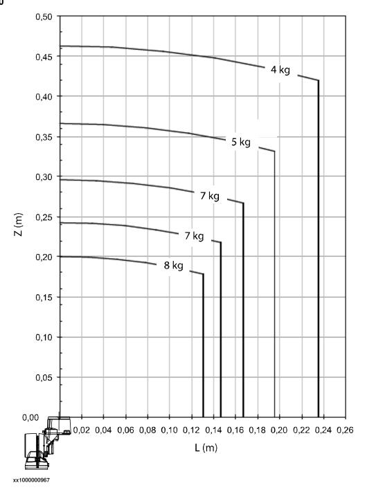
Extra load of 15 kg at the upper arm housing and 1 kg at wrist included in the load diagram.
