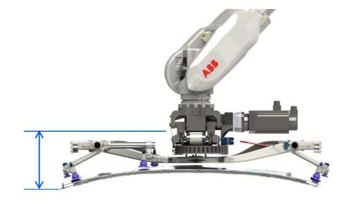
The carbon fiber tooling increases output thanks to its shape design which has been optimized for tool height.
