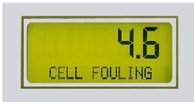
Cell Fouling Alarm Indication
