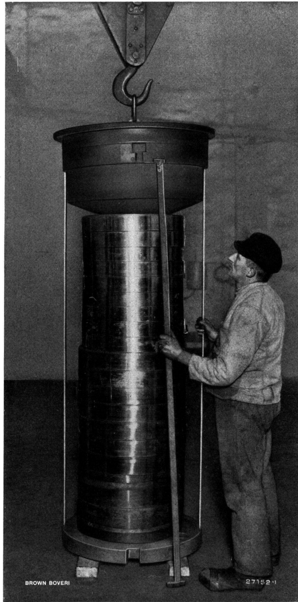
Fig. 5. — Charge of hoop iron on supporting tray. Fixing the suspension rods.
