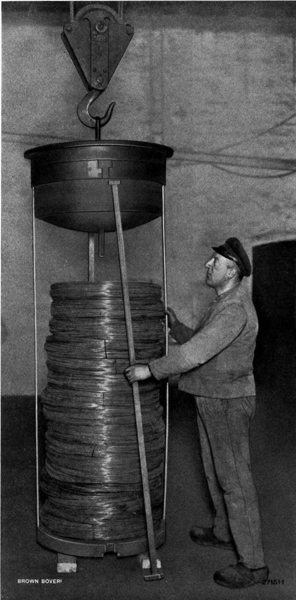
Fig. 4. — Charge of wire coils on supporting tray. Fixing the suspension rods.
