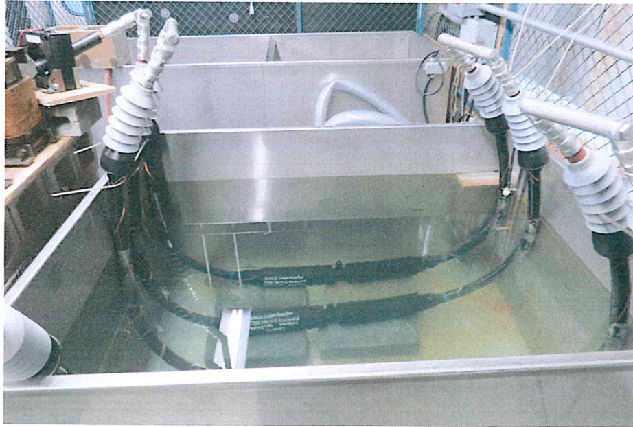
Figure showing water submerged after four hours of heating with current.
