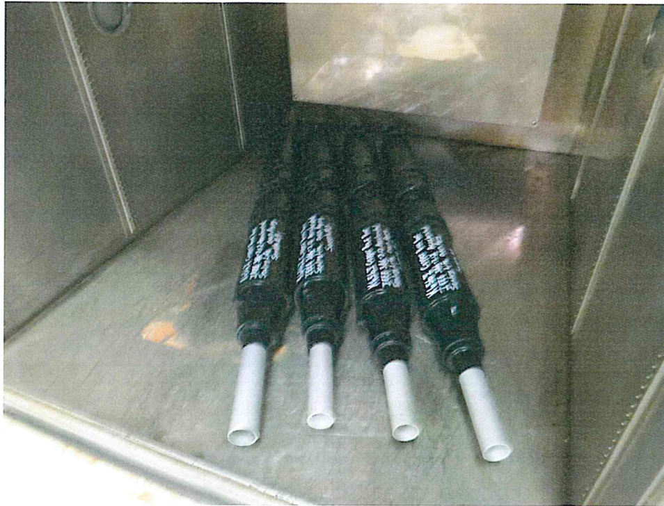
Figure showing four samples of the K676I bus bar with mating parts for oven aging.
