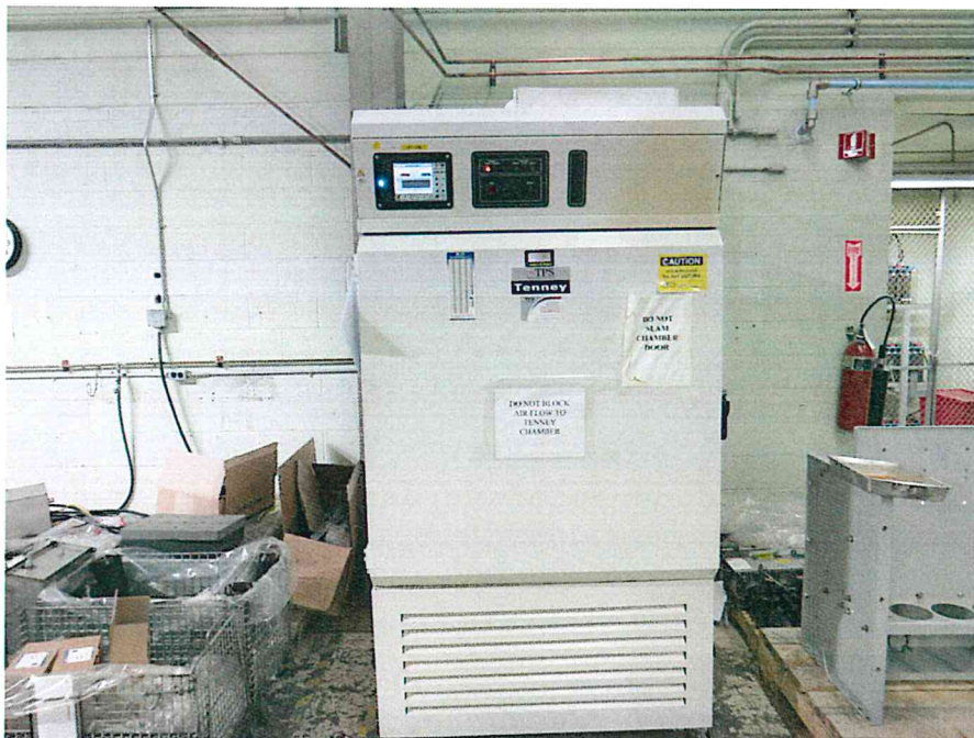
Figure showing the Tenny environmental test chamber.
