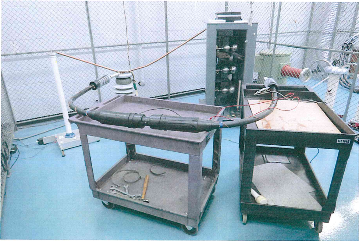
Figure showing impulse test after cycling for sealing life test.
