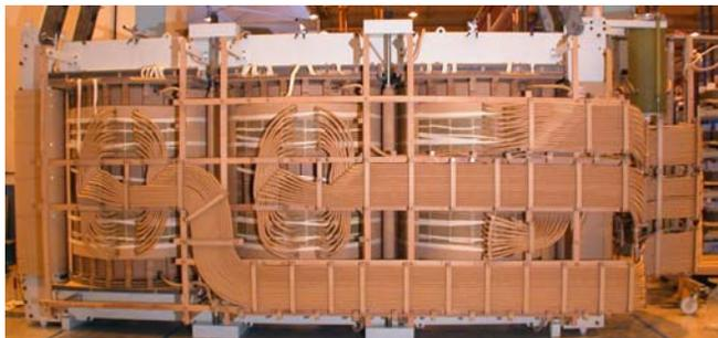
*Figure 4: Active part of a 420 kV/90-200 Mvar VSR*
