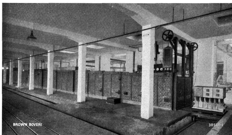
Fig. 53. — Electric twin tunnel-type furnace, for firing and glazing ceramic material, up to 1300^{\circ}\text{C} . Intake 180 kW.
