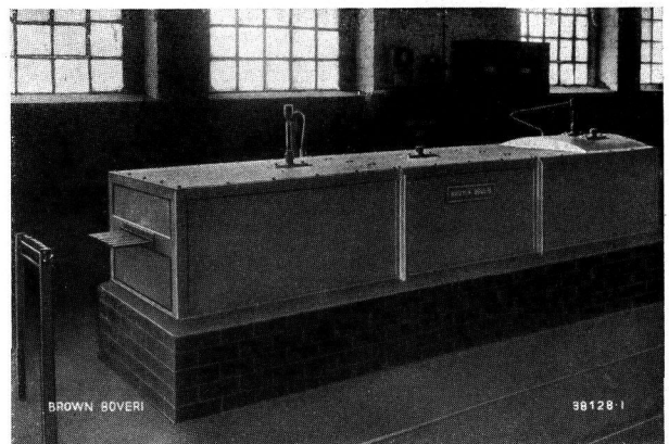
Fig. 57. — Electric wire-drawing furnace for reheating and patenting 12 steel wires in continuous movement at temperatures up to 950° C. Intake 18 kW, automatic temperature regulation.
