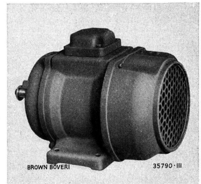
Fig. 3. — Three-phase squirrel-cage motor, with ball bearings, type MUe 34a, completely enclosed with external fan cooling, 1.85 kW, 1500 r.p.m.
