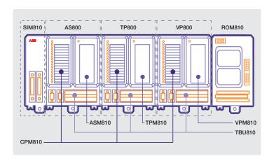
There are also a number of additional common modules which when added to the TP800, VP800 or AS800 products, expand their capability in the following ways:
