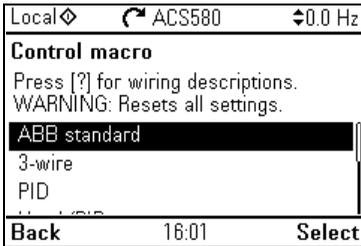
Use the **Macro** submenu to quickly set up drive control and reference source by selecting from a set of predefined wiring configurations.
