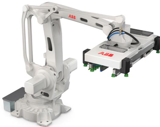
The FlexGripper - Vacuum is a simple plug-and-play extension to the ABB IRB 460 or IRB 660 palletizing robots. For maximum palletizing efficiency, the gripper can handle 40 kilograms and up to 10 products at the same time.
