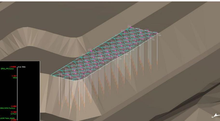
MineScape Drill & Blast provides surface mining drill and blast engineers with an interactive 3D environment in which an optimal blast pattern can be quickly laid out, blast holes projected and charged, blast holes exported for survey, and consumables reported quickly and easily.
