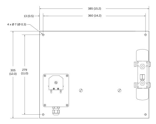
Mounting dimensions – reagent feed pump
