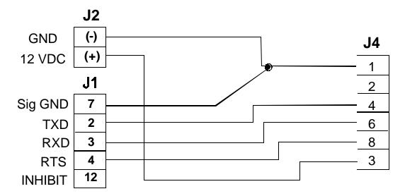
Modifications required to completely duty cycle MDS-2310 with FCU battery power. Can only be wired this way if MDS 2310 has internal 4800 baud modem with part # 031831 AO2 or 031831A11. Advantage: Will reduce radio current consumption by 10-15 milli-amps. Part number is located on the modem board along with the Revision level.
