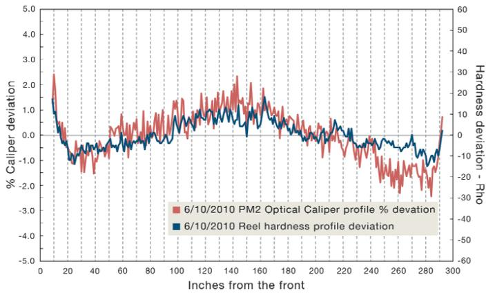
Figure 1 – Profile correlation between Optical Caliper and handheld hardness instrument
