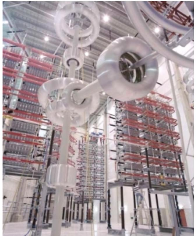
Fig. 3. Capacitor banks of the voltage section
