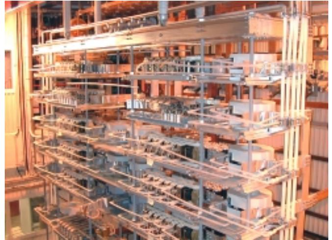
Fig. 2. View of six-pulse back-to-back bridges and test object
