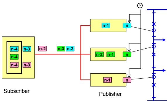
**Figure 7:** The approach to transmit sampled values
