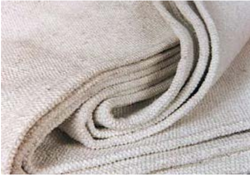
Photo 5 Asbestos Fire Blanket
