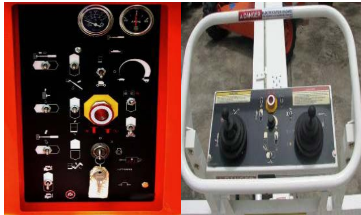
Figs 7 & 8 Example of Ground and Basket controls
