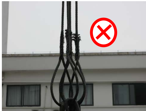
Fig 13 Lifting Slings in Poor Condition
