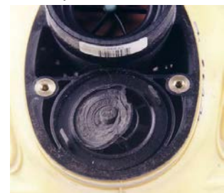
Fig 7 Example of a badly perished valve
