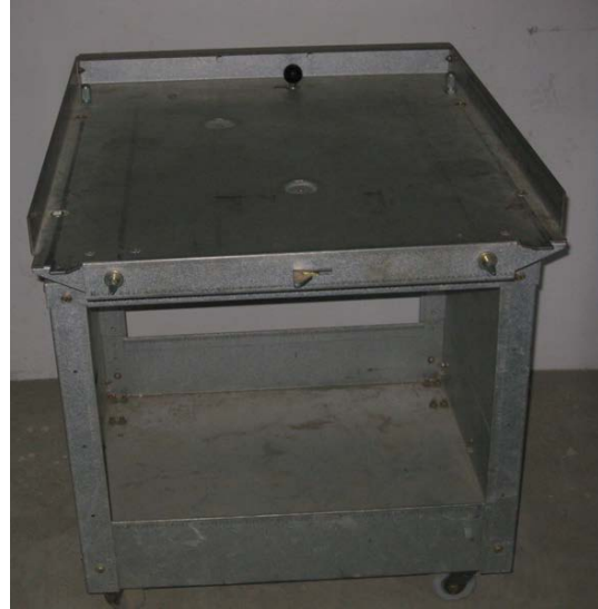
Fig 13 Circuit Breaker Trolley
