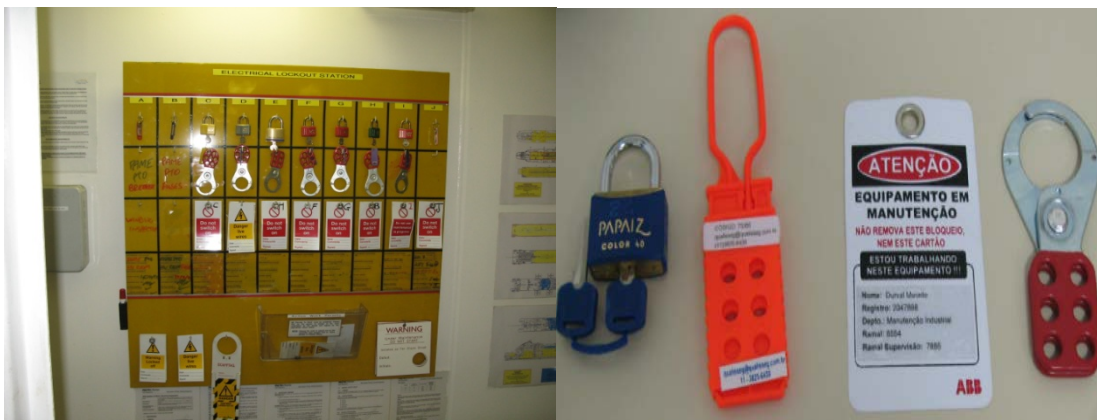
Fig 2 Control of Lock out tag out Equipment Fig 3 Minimum Lock out Tag Out equipment
