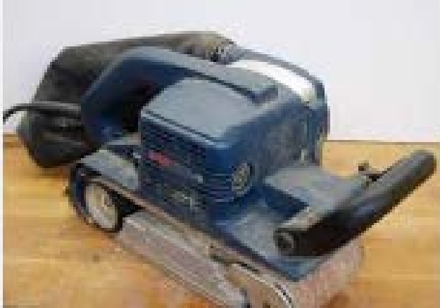
Fig 3 Protection of Nip Point on Belt Sander
