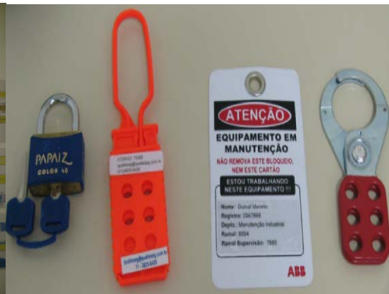
Fig 8 Minimum Lock out Tag Out equipment
