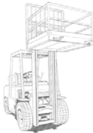
Fig 9 ROLT fitted with a Non Integrated Working Platform
