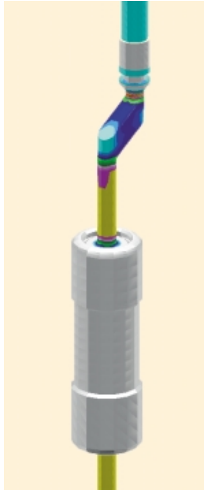
Simulation results showing the loss distribution in one of the phase conductors 6
