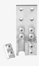
Aluminum lay-in transformer spade connectors feature a slide-out keeper to minimize the hassle and hazards of forcing cables into the closed cable ports found on conventional mechanical connectors — saving time and labor. ZBK series also has a compact Zeebar® design that halves cantilever stress and doubles cable capacity.
