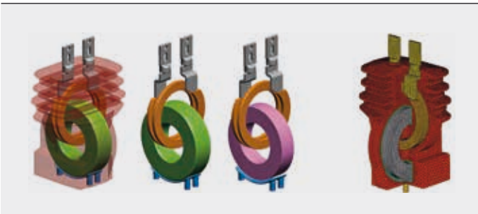
8 Geometry of current transformer (left) and its discretization in ABAQUS (right)
