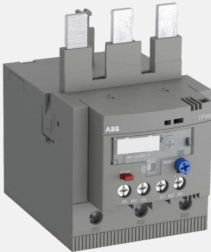
ABB's TF96 thermal overload relays are economic electromechanical protection devices for the main circuit. They are used mainly to protect motors against overload and phase failures. Starter combinations are setup together with contactors.
