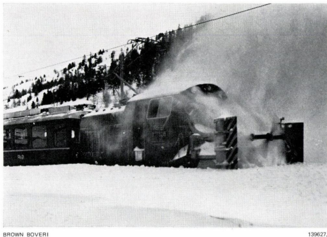
Fig. 4 – Rotary snowplough on the Bernina section
