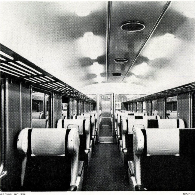
Fig. 3 – Arrangement of fluorescent lights in the passenger area of a Type II (A) standard coach of Swiss Federal Railways
