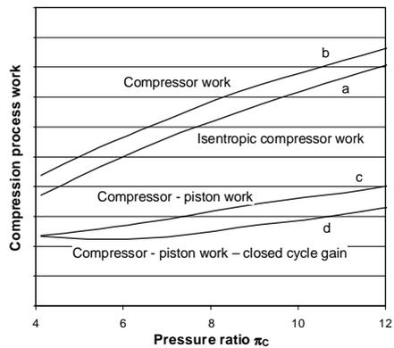
Fig. 7 Compressor work versus  $\pi_c$
