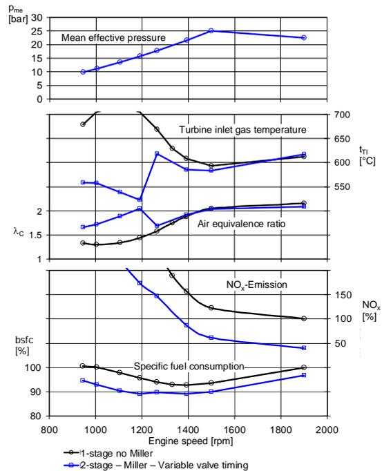
Fig. 18: Improved torque capacity with 2-stage turbocharging
