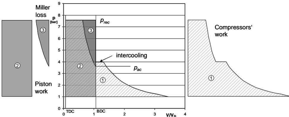
Fig. 6:  $p$  -  $V$  diagram of the charging process
