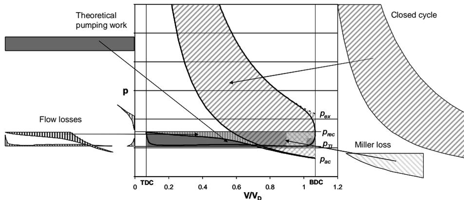
Fig. 9: Complete process analysis
