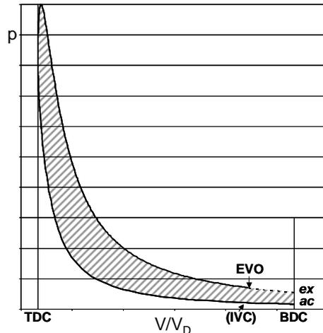
Fig. 1. Pressure – volume diagrams of the closed cycle
