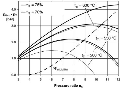
Fig. 13: Pressure difference over cylinder
