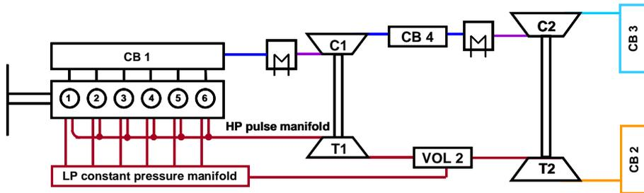
Fig. 4: Two-port pulse system
