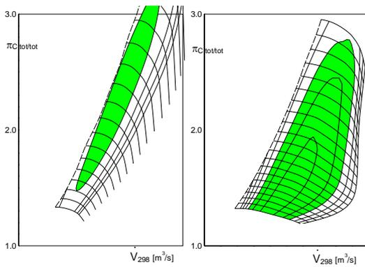
Fig. 15: HP Compressor map vs. standard compressor map (green areas: same efficiency)
