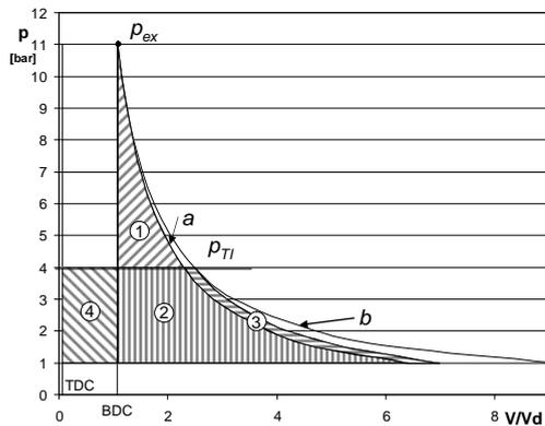
Fig. 3. Pressure – volume diagrams of the exhaust process
