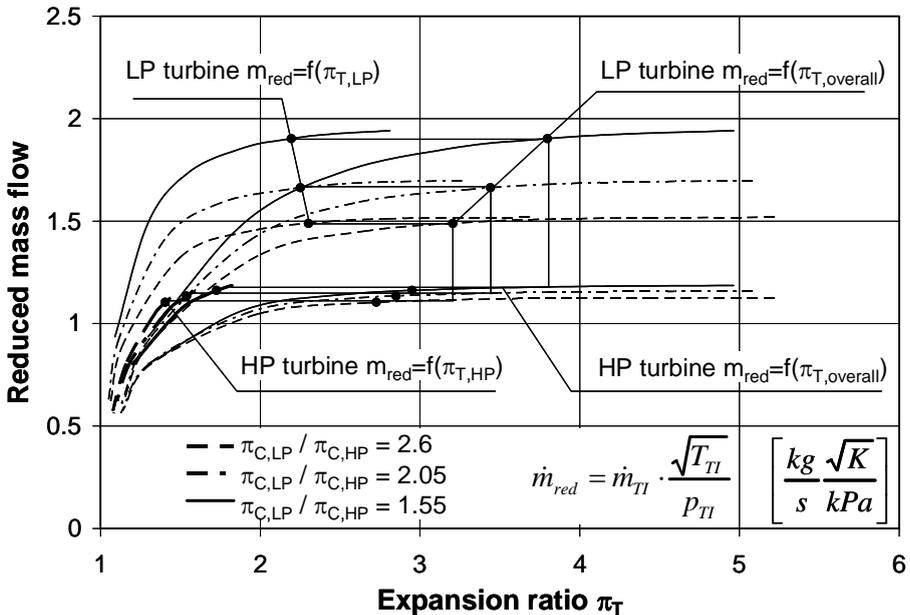
Fig. 12: Flow characteristics
