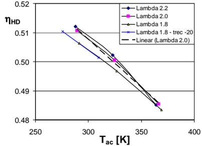
Fig. 2: Closed cycle efficiency over  $t_{ac}$
