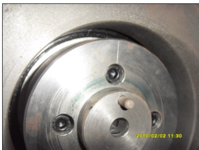
Figure 5: Cylindrical pin attached to the shaft ND-end.
