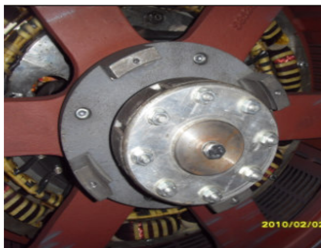
Figure 6: The PMG shaft pressed in and attached with main rotor with the hexagonal M10 screw.
