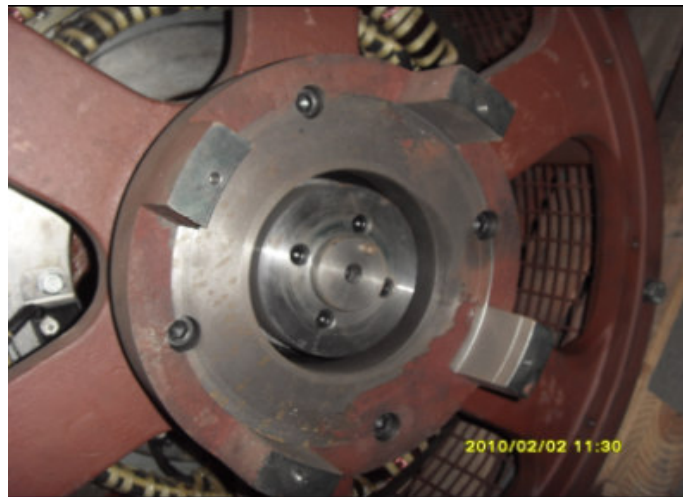
Figure 3: PMG retainer attached to the NDE-shield
