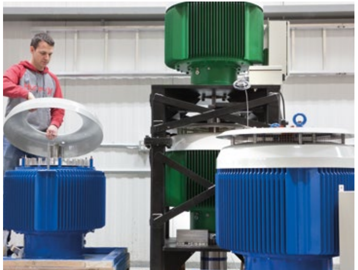
With a MagnoDrive and the appropriate VFD, the full torque envelope is available throughout the entire speed range.
