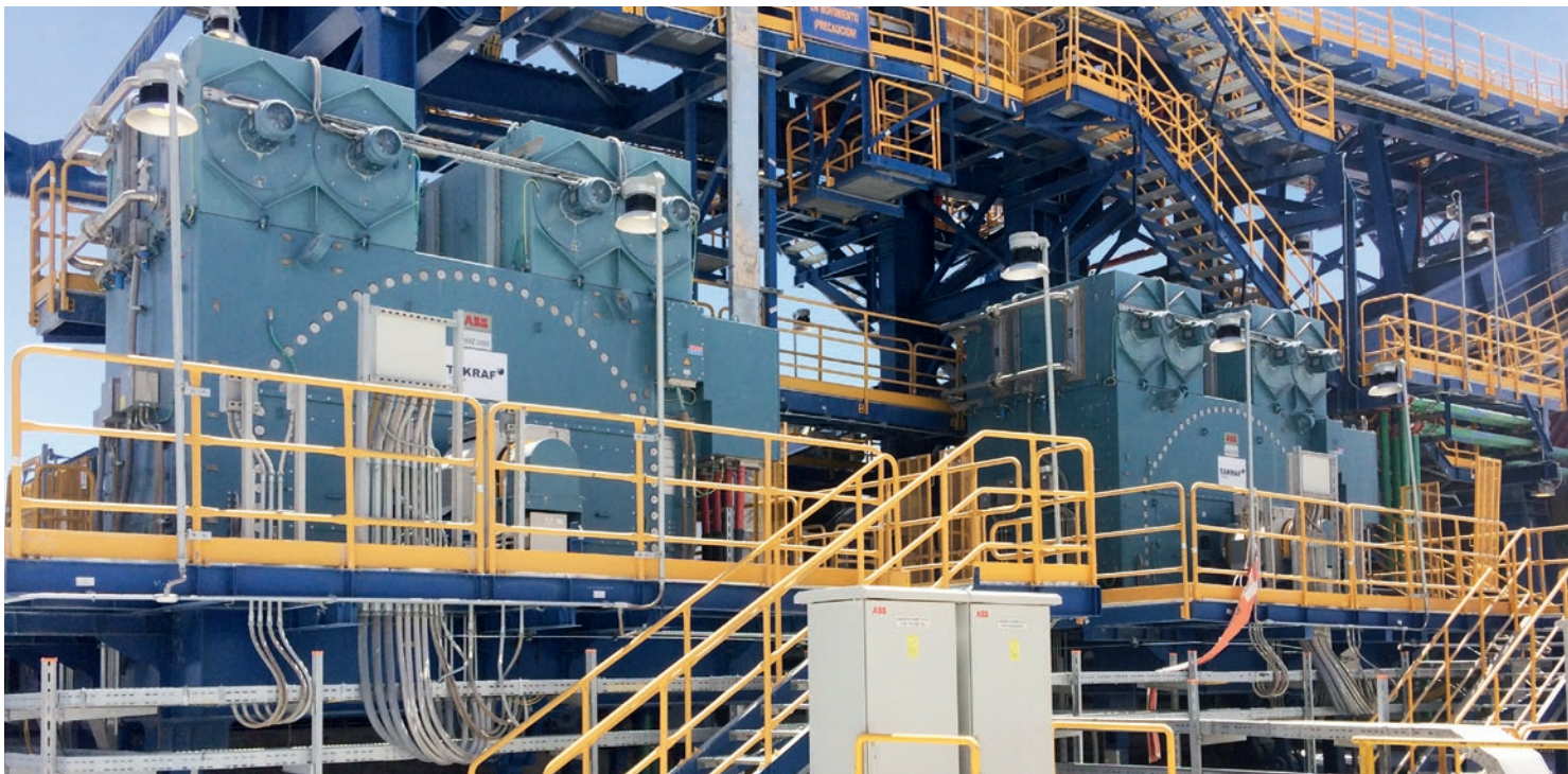
Gearless conveyor drives (GCD) for high power
