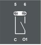
Common, voltage supply | 5                  | 5 A@250 Vac (AC-1), 5 A@30 Vdc |
