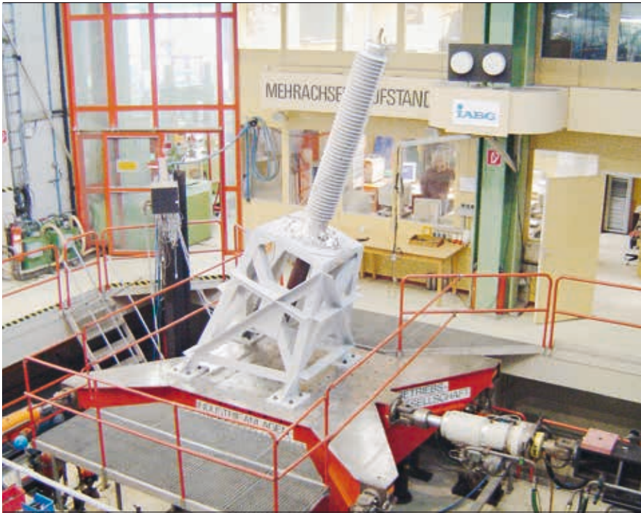
1a RIP 230 kV bushing under seismic test
