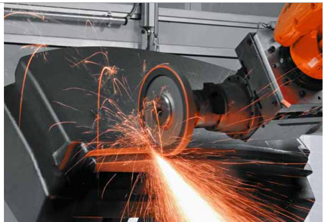
4 Grinding process where the robot slows down when encountering excessive burr. The measured process force exceeds the set reference value, which triggers the robot to slow down. When the force is decreased, the robot will accelerate to the programmed speed in 0.1 s
