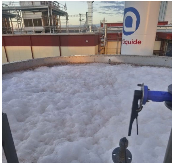
03 Foam in a knockout pot in Oil & Gas industry
