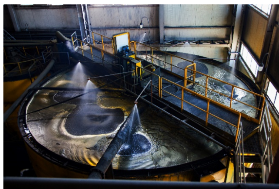
04 Foam in floatation tank in the mining industry
