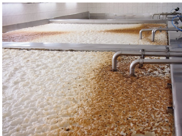
06 Foaming during fermentation in the brewing process
