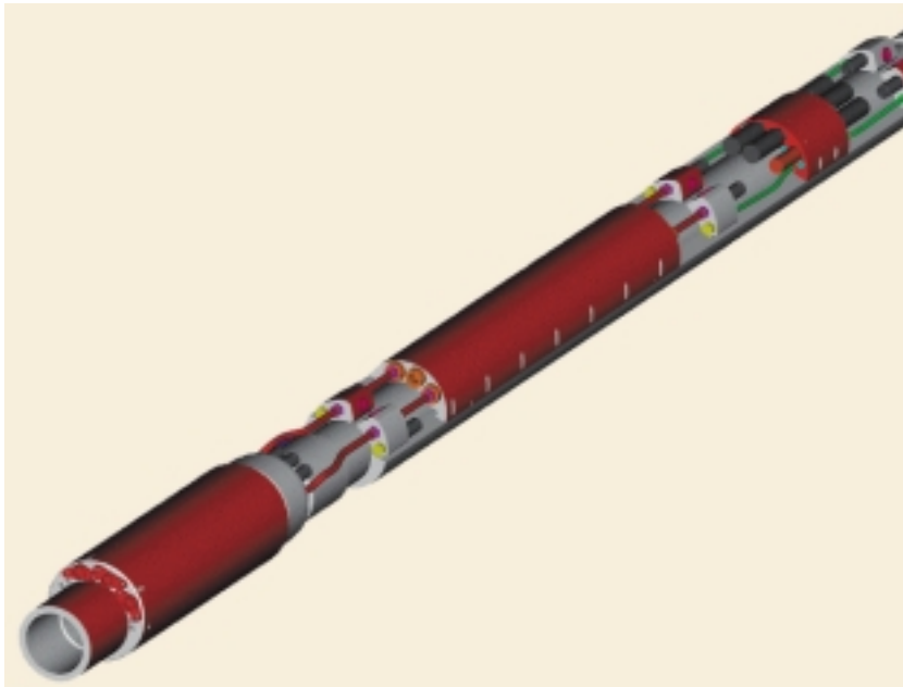
2 A 3D model of a downhole choke showing how the various functions are stacked on the outside of the flow-path
